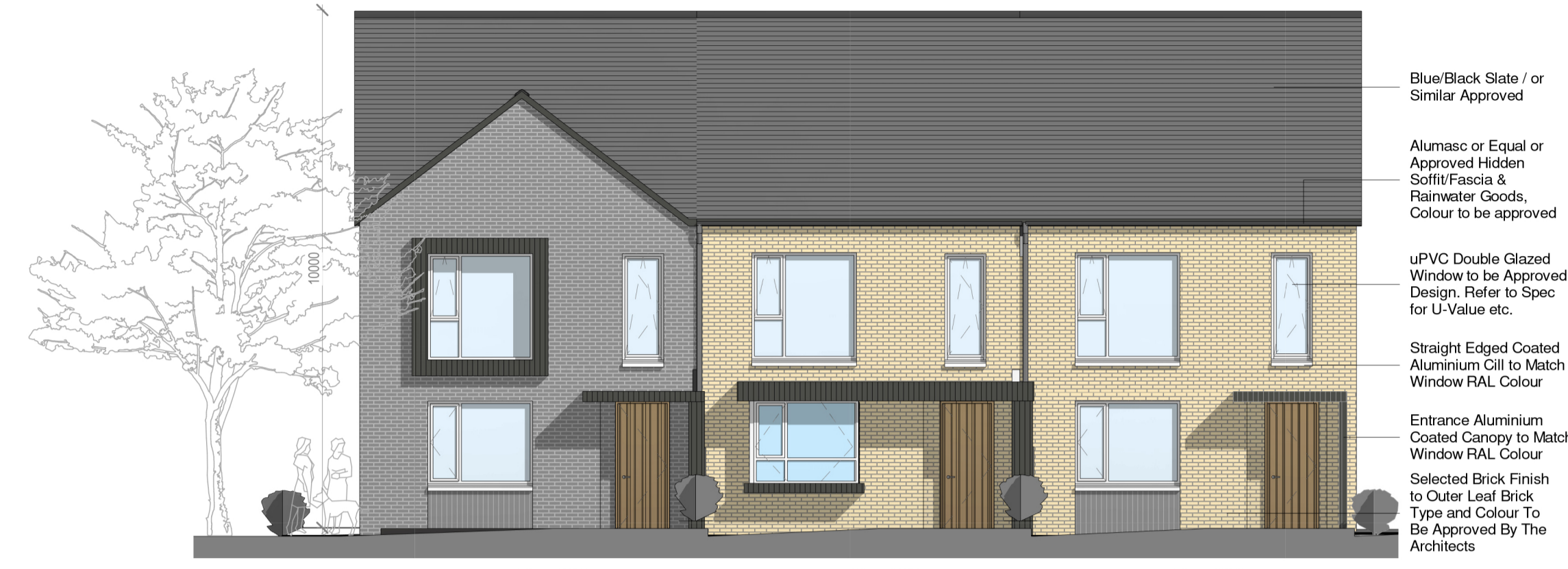
3 Block 3.1 - Front Elevation 1:100
