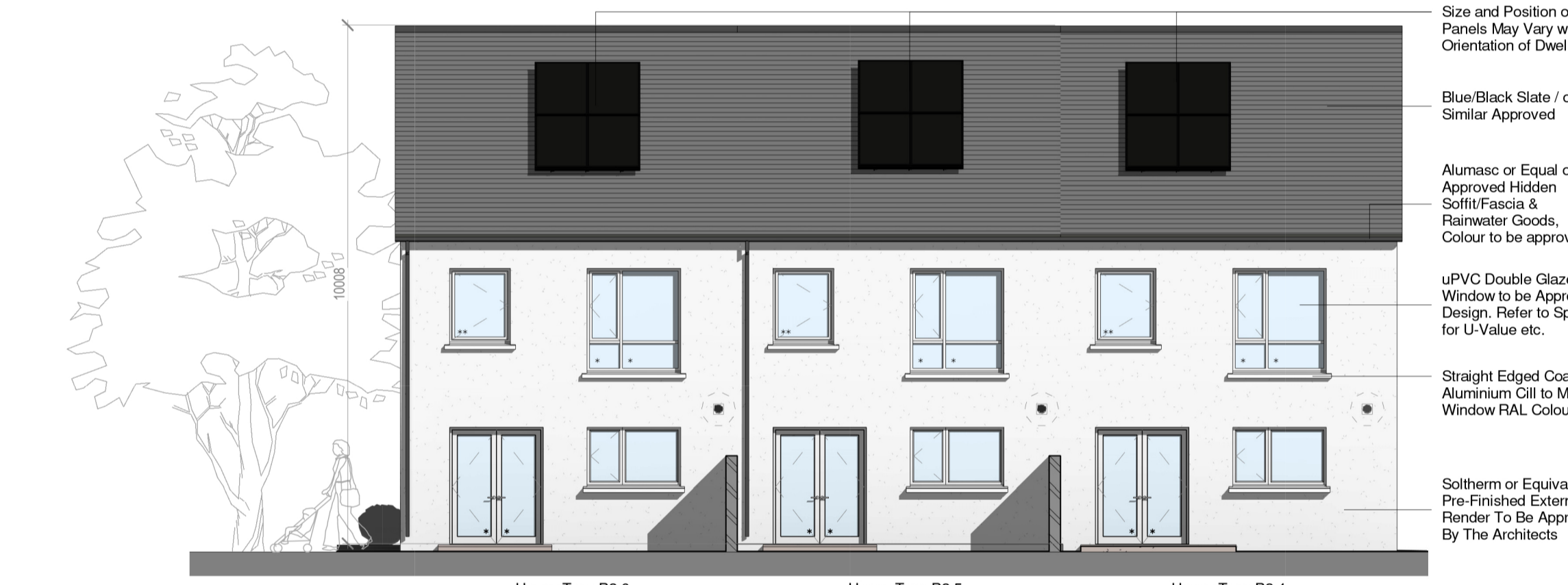
4 Block 3.1 - Rear Elevation 1:100
